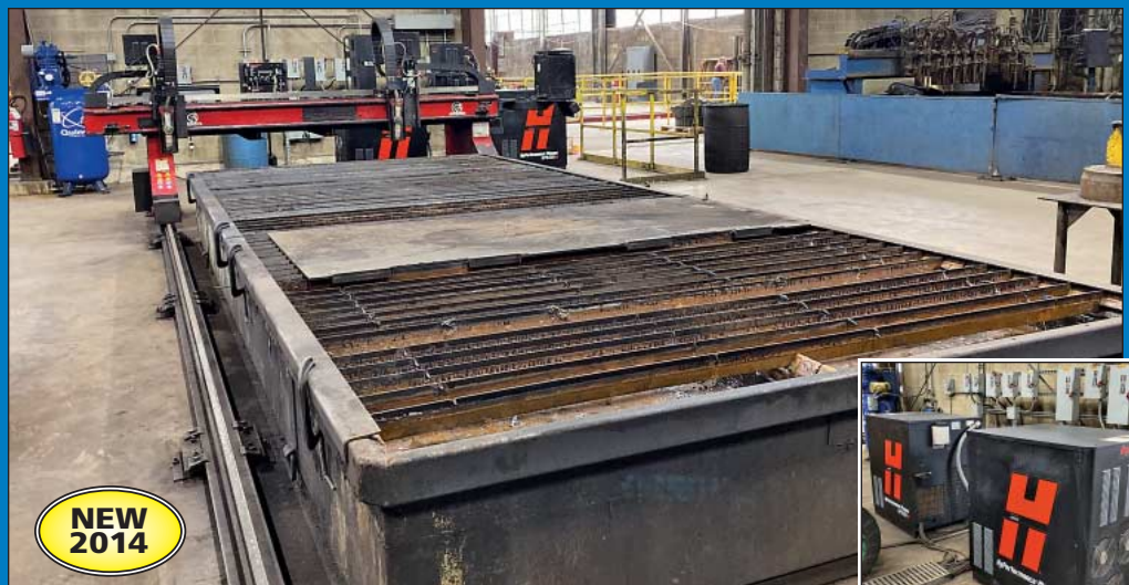
9' x 20' Cutting Systems Raptor Two-Torch CNC Plasma Table w/ (2) 260-Amp Hypertherm Power Supplies
