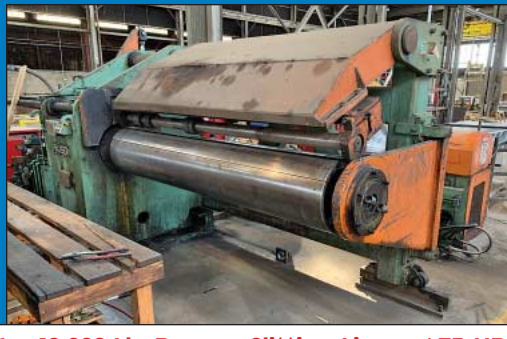
.100 x 106" x 40,000 Lb. Paxson Slitting Line w/ 75-HP Recoiler
